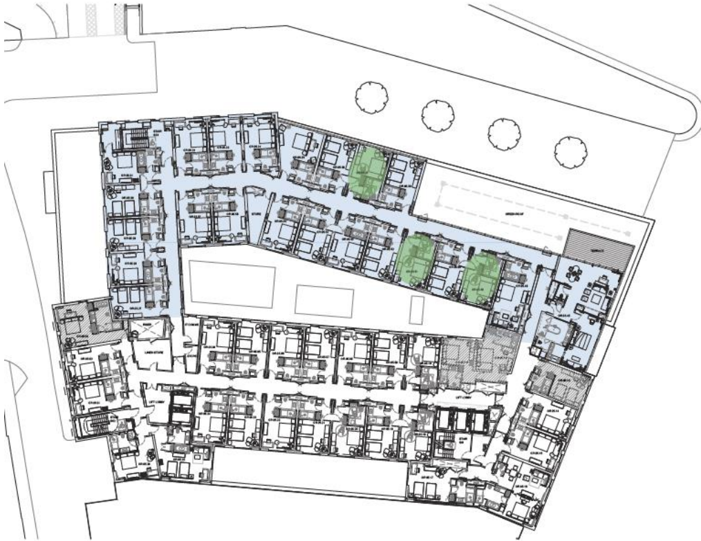
Image 3: Proposed fifth floor plan. The blue shading refers to the proposed extension, the green demarcates the proposed accessible guestrooms and the grey shading is the existing building.
